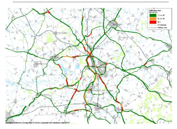
Figure 10: Highway Network in the morning peak – volume of traffic in relation to road capacity (85% to 95% = at capacity, 95% plus = over capacity)
