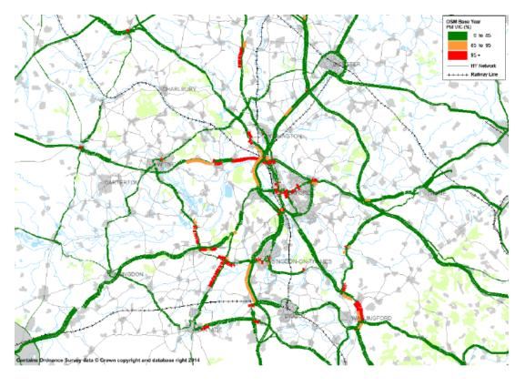
Figure 11: Highway Network in the evening peak – volume of traffic in relation to road capacity (85% to 95% = at capacity, 95% plus = over capacity)
