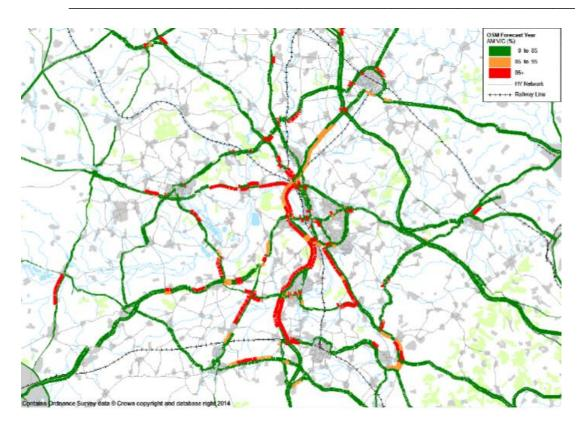
Figure 15: Highway Network in the morning peak in 2031 with no intervention – volume of traffic in relation to road capacity (85% to 95% = at capacity, 95% plus = over capacity)
