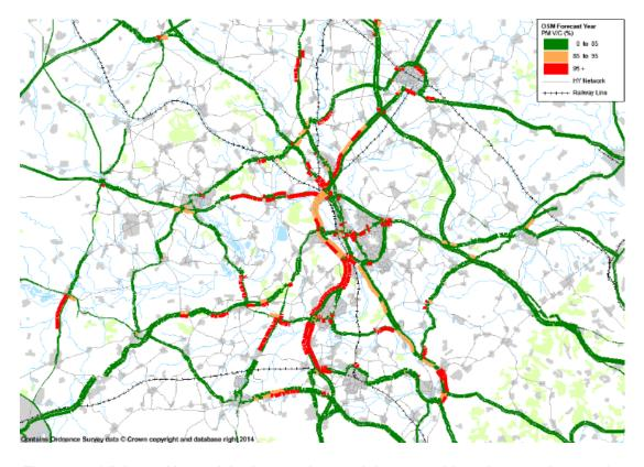
Figure 16: Highway Network in the evening peak in 2031 with no intervention – volume of traffic in relation to road capacity (85% to 95% = at capacity, 95% plus = over capacity)
